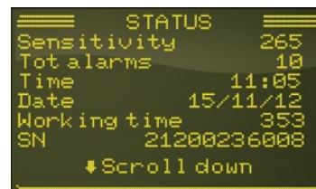
Display of the status of the metal detector
